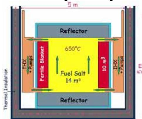
Fig.1. Schematic vertical section of the TMSR, including pumps and heat exchangers (IHX)
