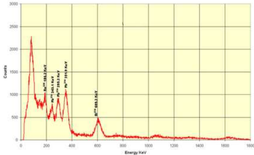
Figure 20. Gamma ray spectroscopy of typical oxidized uranium ore sample; Ra-226, Bi-214 and Pb-214 are well defined (Kind permission of Stratamodel Professional Geologic Services) 185 .
