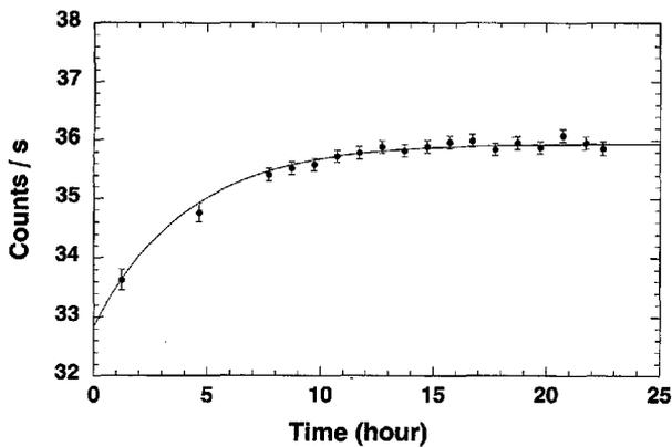
Fig. 4 Growth curve of the 0.605 MeV  $\gamma$ -ray emitted from the ground state  $^{134g}\text{Cs}$
