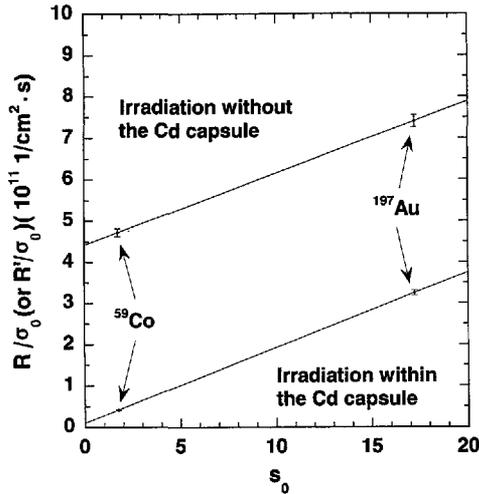
Fig. 5 Experimental relation between  $R/\sigma_0$  (or  $R'/\sigma_0$ ) and  $s_0$  obtained by flux monitor wires irradiated without and within the Cd shield capsule
