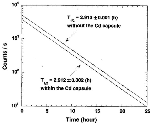
Fig. 3 Decay curves of the 0.127 MeV  $\gamma$ -ray emitted from the isomeric state  $^{134m}\text{Cs}$
