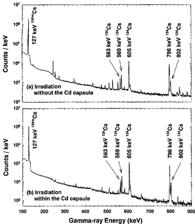
Fig. 1 Gamma-ray spectra of Cs targets irradiated (a) without and (b) within the Cd shield capsule by reactor neutrons
