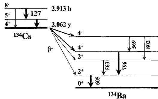
Fig. 2 A partial decay scheme of  $^{134}\text{Cs}$
