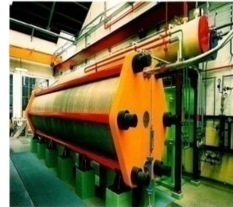
Pressure electrolyzer (Lurgi System) for hydrogen production, capacity 700 Nm 3 /h H 2
