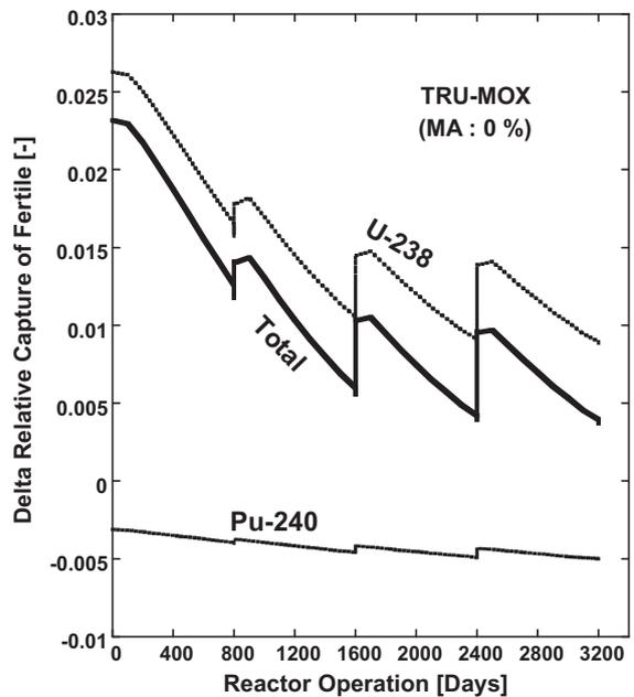
Fig. 14. Relative capture fertile rate of compared MOX with TRU fuels for no doping case.
