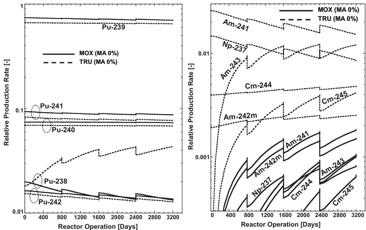
Fig. 9. Relative production rate of MOX and TRU fuels for no doping case.
