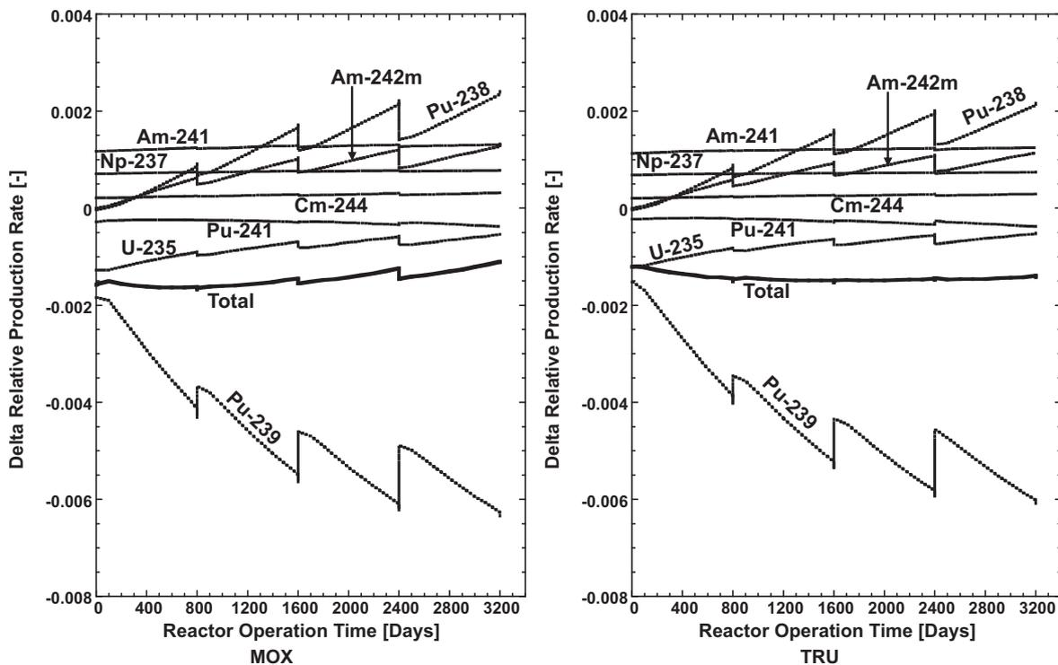
Fig. 11. Delta relative production rate of compared MOX and TRU for no MA doping case with MA doping case.
