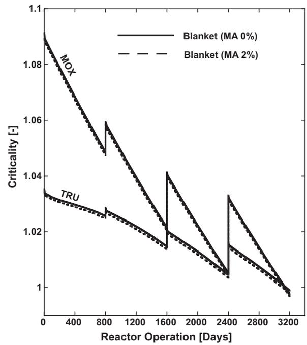
Fig. 7. Reactor criticality of MOX and TRU fuels for no doping and with doping MA cases.
