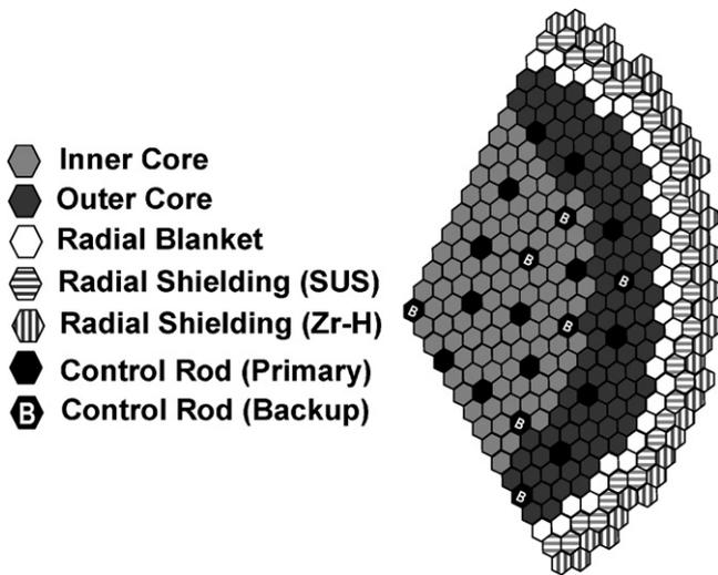
Fig. 2. Configuration of reactor core (1/3 scale).
