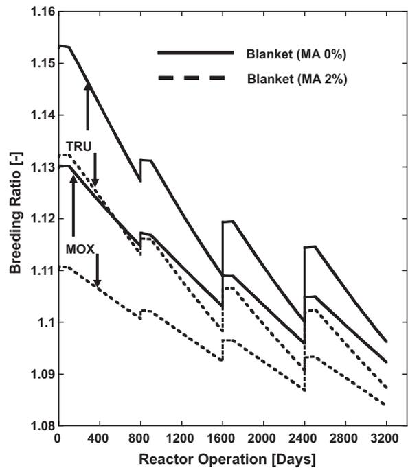
Fig. 12. Breeding capability of MOX and TRU fuels for no doping and with doping MA.
