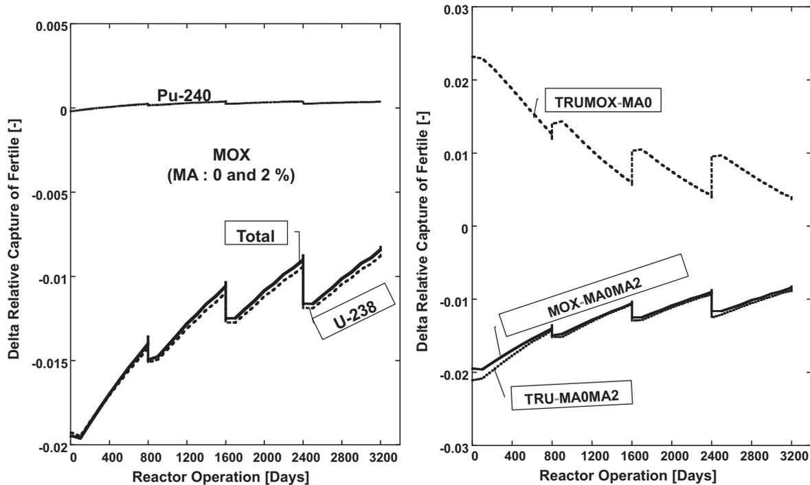
Fig. 15. Delta relative capture fertile rate of MOX and TRU fuels for no MA doping and with MA doping cases.
