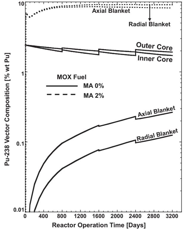
Fig. 18. Isotopic plutonium vector composition of MOX and TRU fuels.
