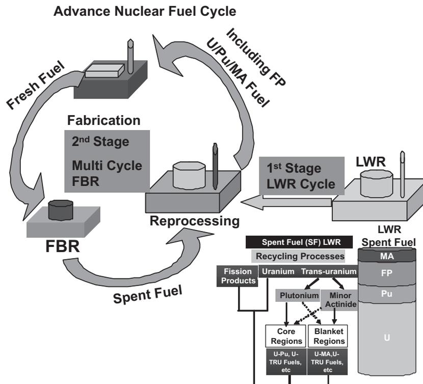
Fig. 1. Advance nuclear fuel cycle scheme.
