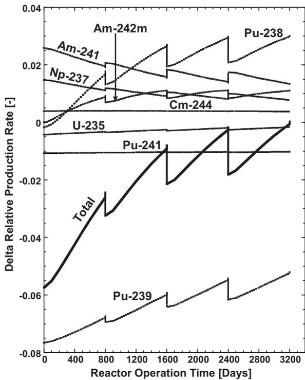
Fig. 10. Delta relative production rate of compared MOX with TRU fuels for no doping.
