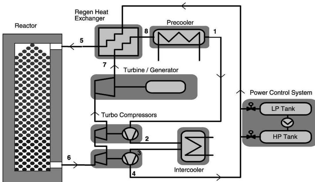
Figure 12 Simplified diagram of the PBMR Brayton cycle system [101]
