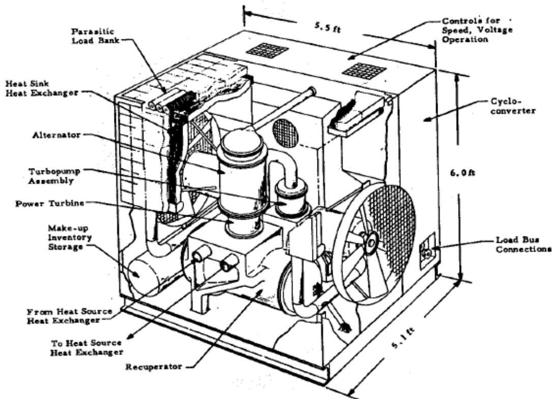
Figure 9 Sketch of the Feher 150 kWe S-CO<sub>2</sub> power cycle [37]
