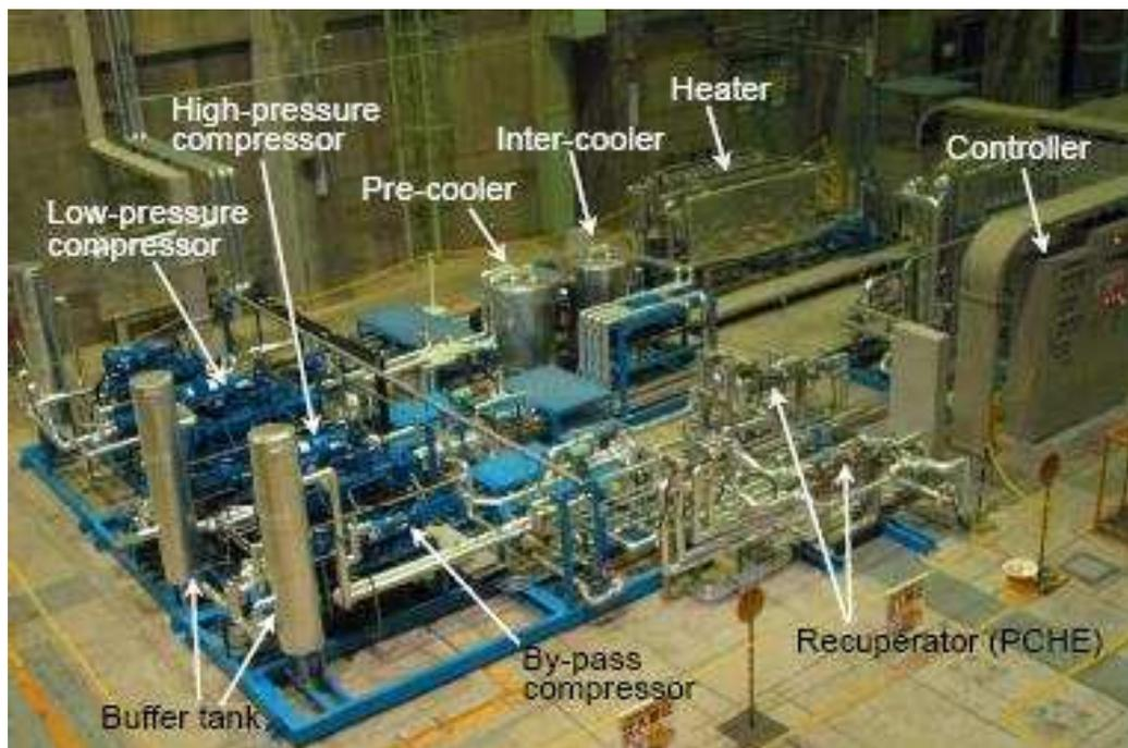
Figure 14 JAEA S-CO<sub>2</sub> cycle test loop [106]
