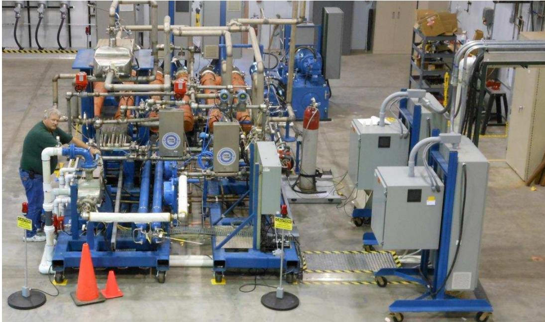
**Figure 15 S-CO<sub>2</sub> split flow recompression CBC test assembly at SNL (Courtesy of SNL)**
