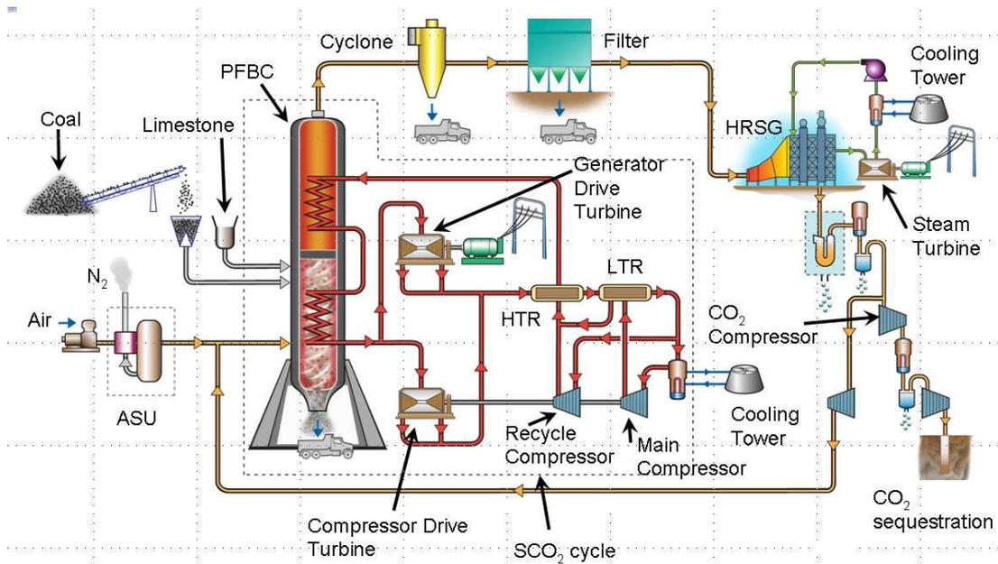
Figure 5 AR's oxy-combustion coal-fired S-CO<sub>2</sub> Brayton cycle [47]
