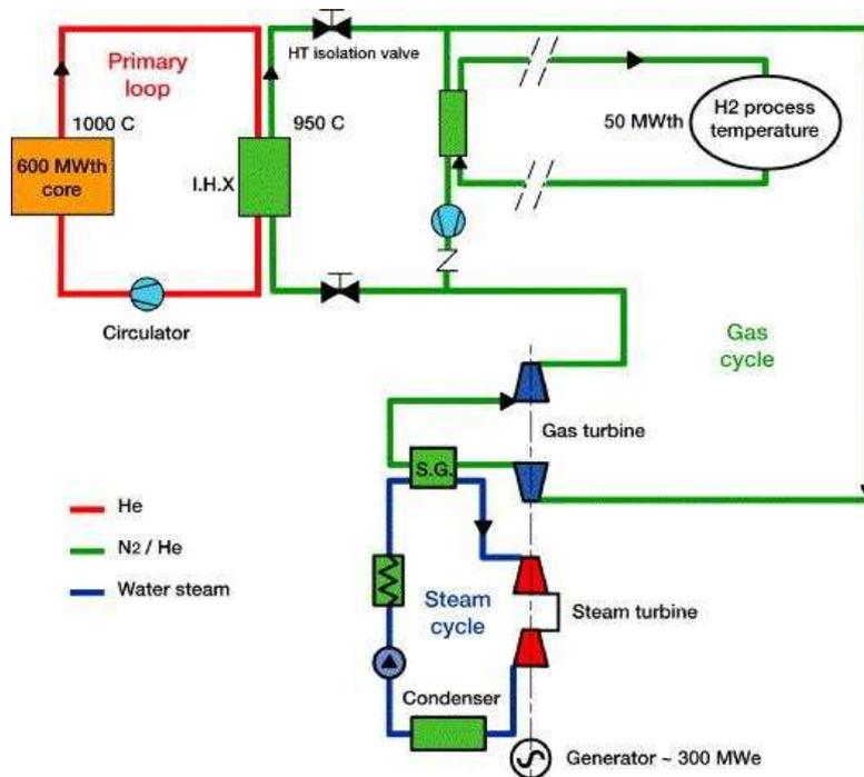
Figure 17 Schematic of the V/HTR ANTARES plant [31]
