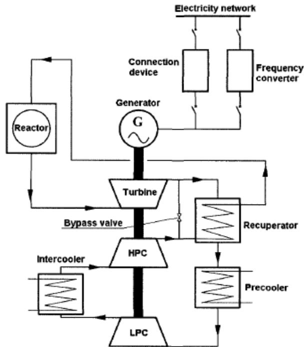
Figure 16 Schematic of HTR-10GT [30]
