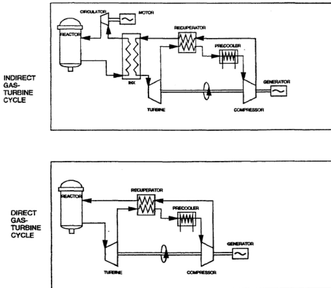
Figure 6 Indirect and direct nuclear GT cycles [57]
