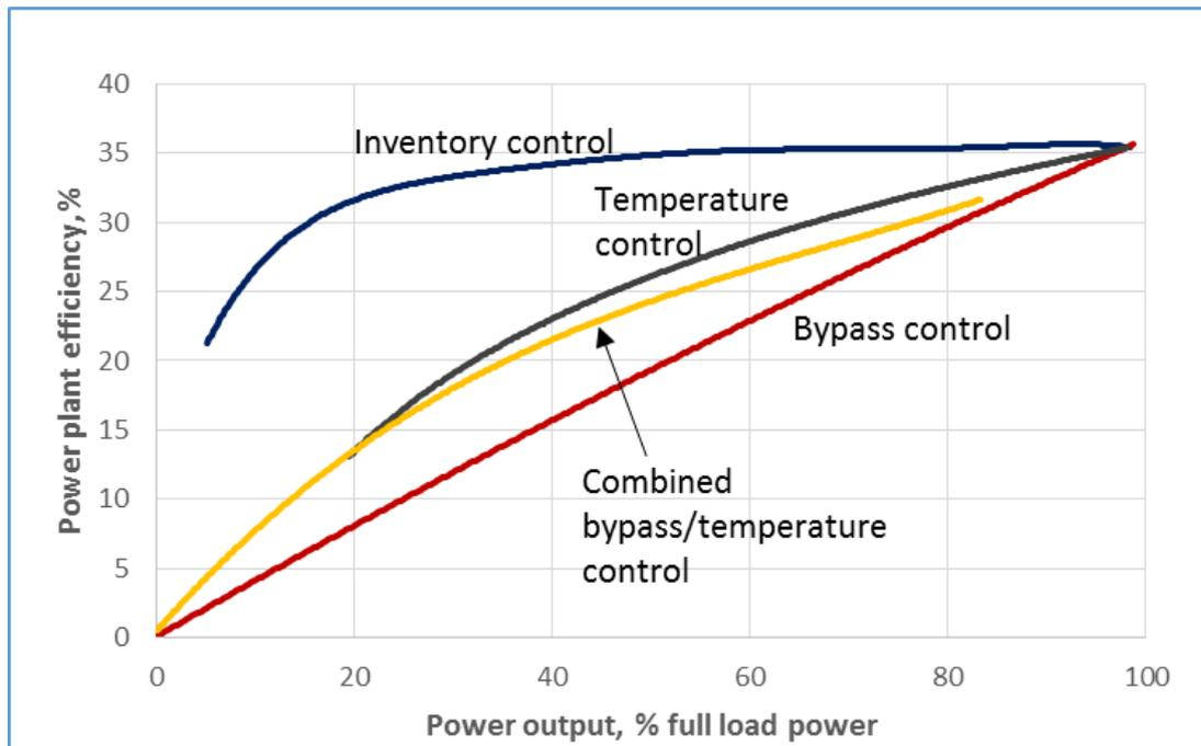
**Figure 19** Effect of different control scheme on cycle efficiency
