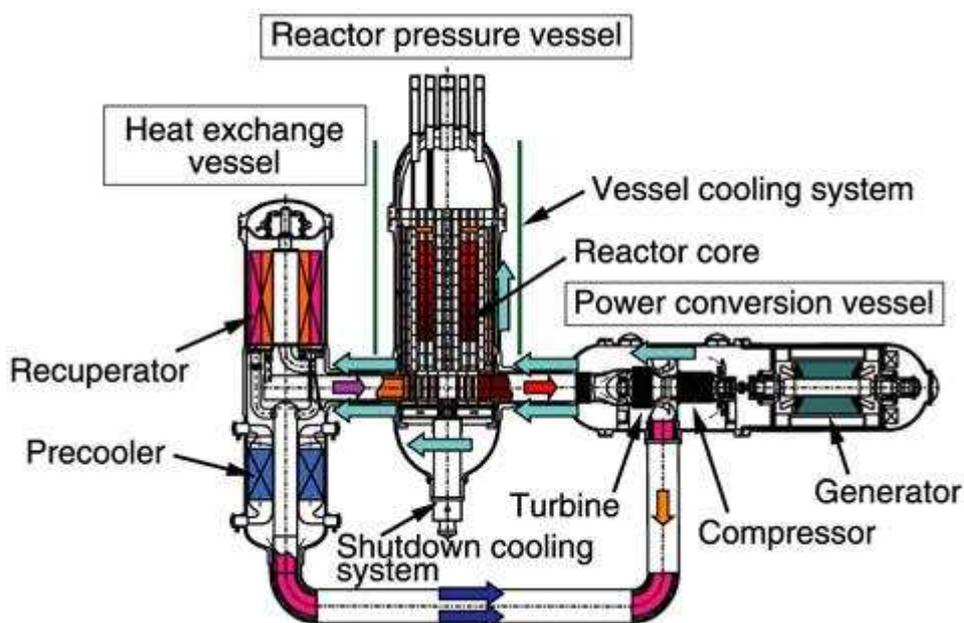
Figure 13 Layout of GTHTR300 (Courtesy of JAERI)
