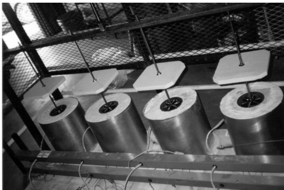
Figure 1. Crucible furnaces and mechanical cycling frame used to evaluate corrosion in molten nitrate salt during thermal cycling. The fixtures for the stainless steel coupons are visible at the top of the crucibles.
