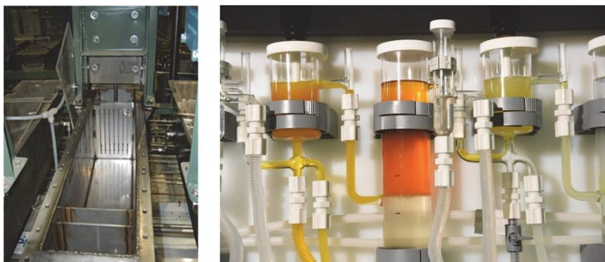
**Figure 3.** Industrial and lab-scale mixer-settlers.
