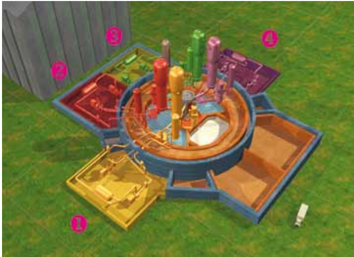
Fig. 1.2-8 Four Train Concept and corium spreading area
