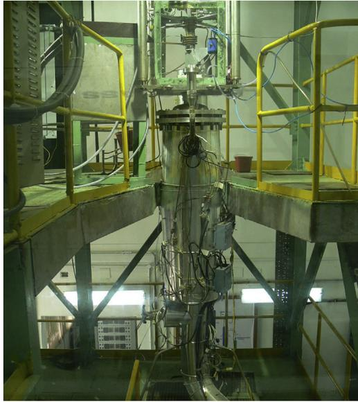
**Figure 15.23** Sodium-Fuel Interaction Facility (SOFI): Facility for molten fuel interaction studies.
