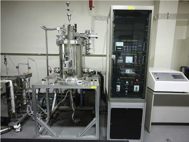
**Figure 13.15** TRISO coating system.
