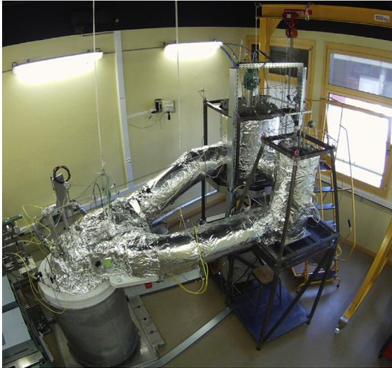
**Figure 7.19** Completed loop with its thermal insulation.
