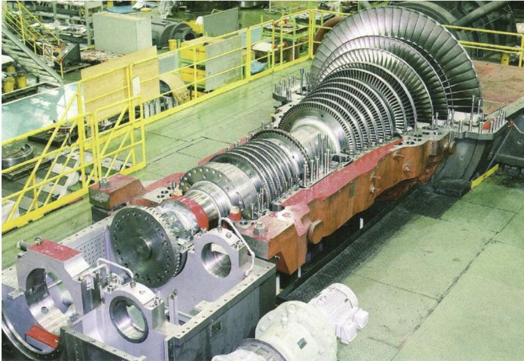
**Figure A1.3** Photo of combined cycle power plant steam turbine with open cover (courtesy and copyright of MHI). Single-cylinder reheat turbines are used.
