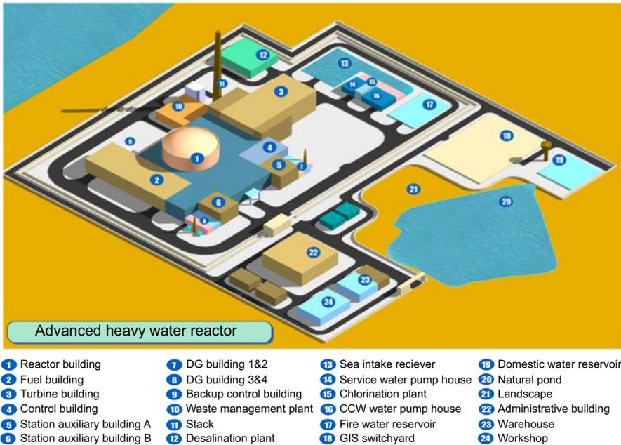
**Figure 15.4** Advanced heavy water reactor plant layout.
