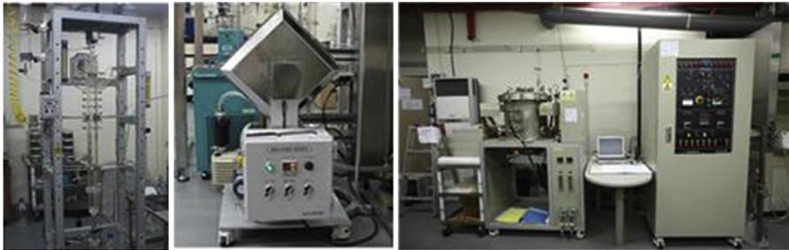
Figure 13.13 Kernel fabrication system.
