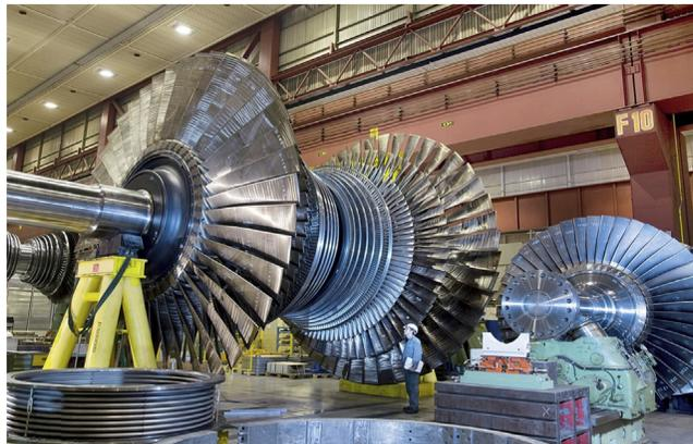
**Figure A1.7** Photo of LP double-flow steam turbine rotor with blades for supercritical pressure coal-fired power plant.
