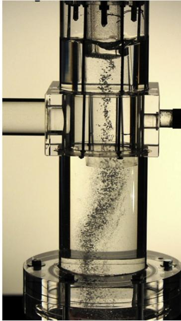
**Figure 7.20** Water mock-up of the separator showing the concentration of bubbles in the vortex center and their coalescence. The gas is evacuated at the top and the liquid through the pipe on the left.
