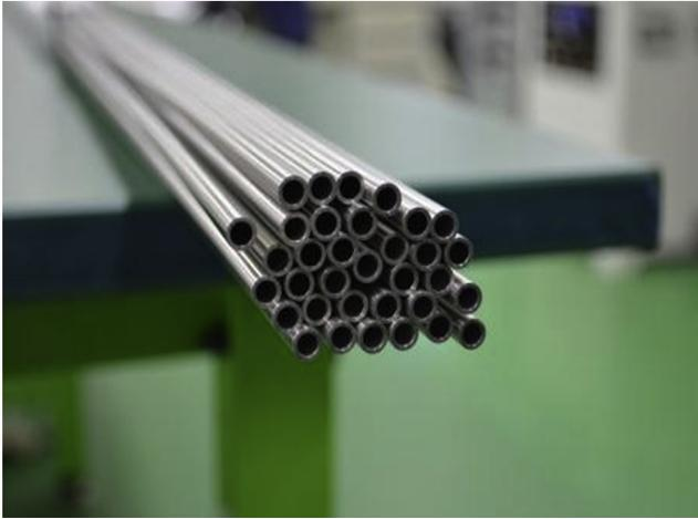
**Figure 13.9** FC92 cladding tubes.
