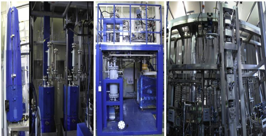
Figure 13.18 50 NL·H<sub>2</sub>/h-scale SI test facilities.
