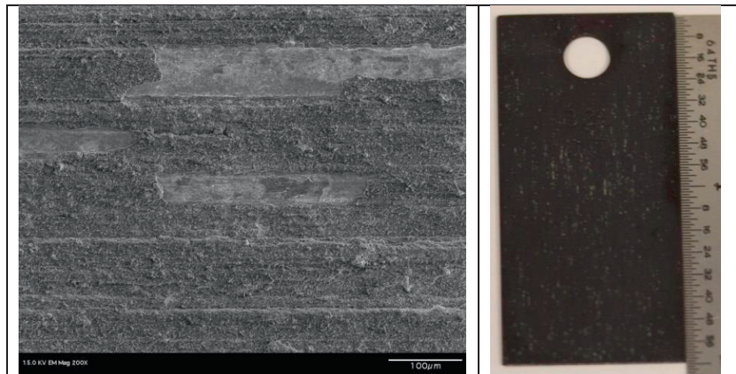
Figure 3: Plan view of 321SS after at 600°C for 1000 hours (top left image). Observed scaling present in photograph (top right) allowed for visual traces of spallation.
